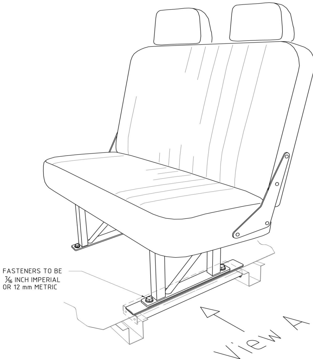
Diagram 2.11(3)(a) Channel spans between structural cross-members
