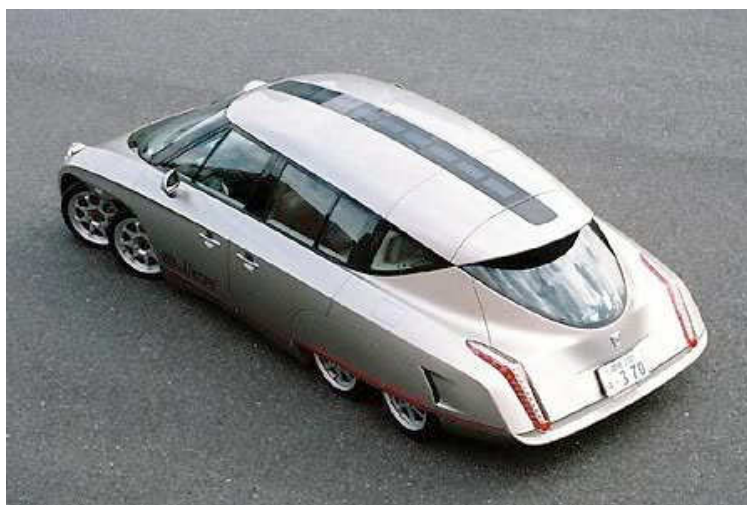
The picture is of the SIM-Drive concept electric Eliica car that can do 0-100 in 4 seconds, 370km/h top speed
