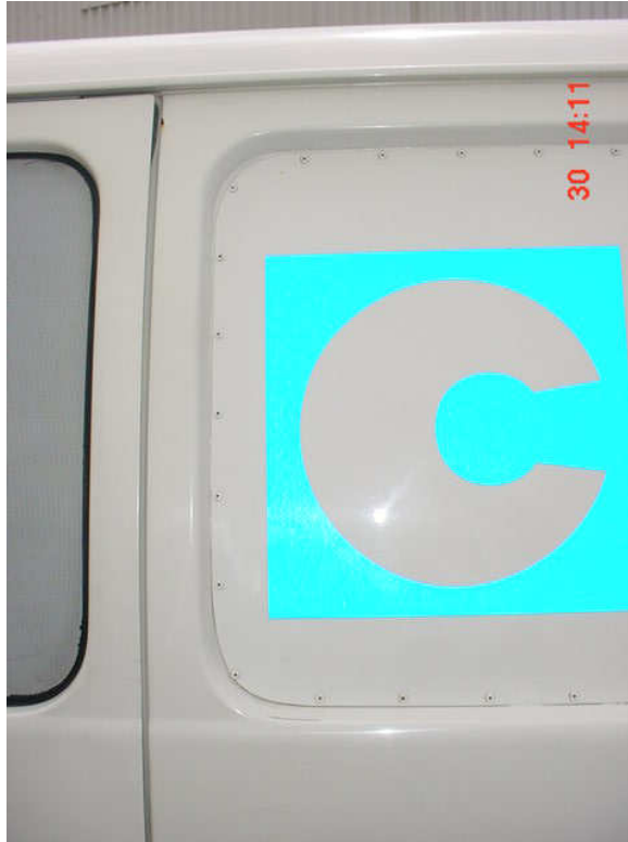
C) This vehicle had two rear side windows; one has been fitted with a metal screen, the other with a riveted blanking plate.
