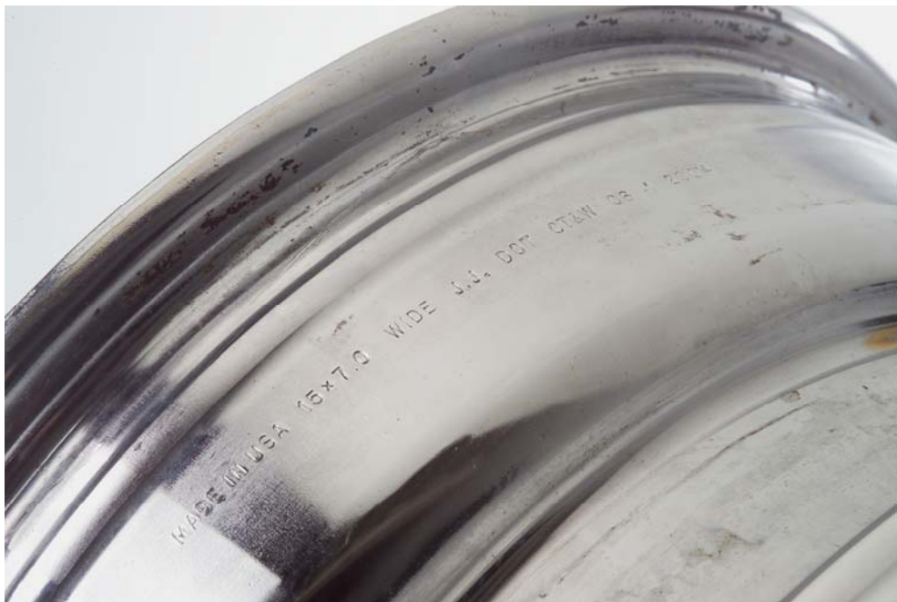
'DOT' compliance marking is evident on rim, but that applies only to the rim itself, not the manufactured wheel.
