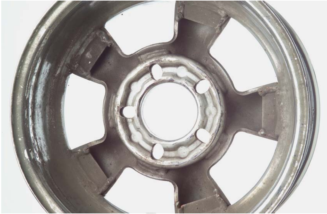
View of back-face of poorly designed and assembled 'Supreme' wheel.
