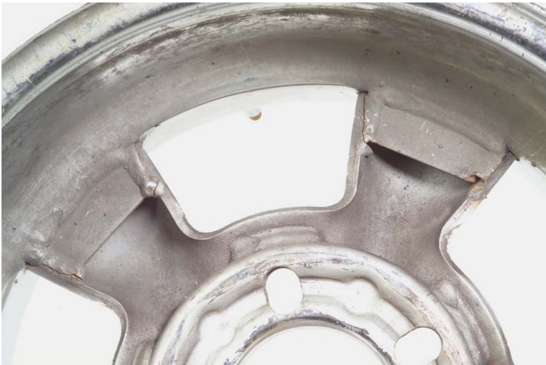
Close-up view of where the weld-lug has been poorly welded to the centre section spokes, and failed.
