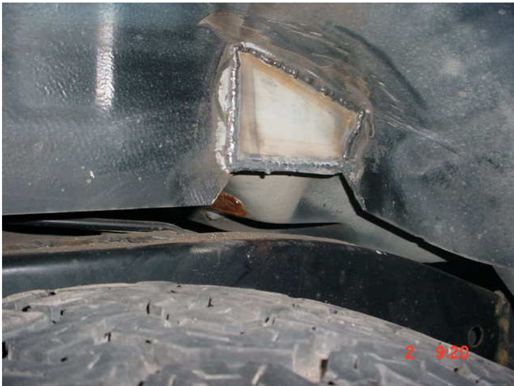
Cut out and patch repair (if necessary), the wheel arch seatbelt anchorage area.
