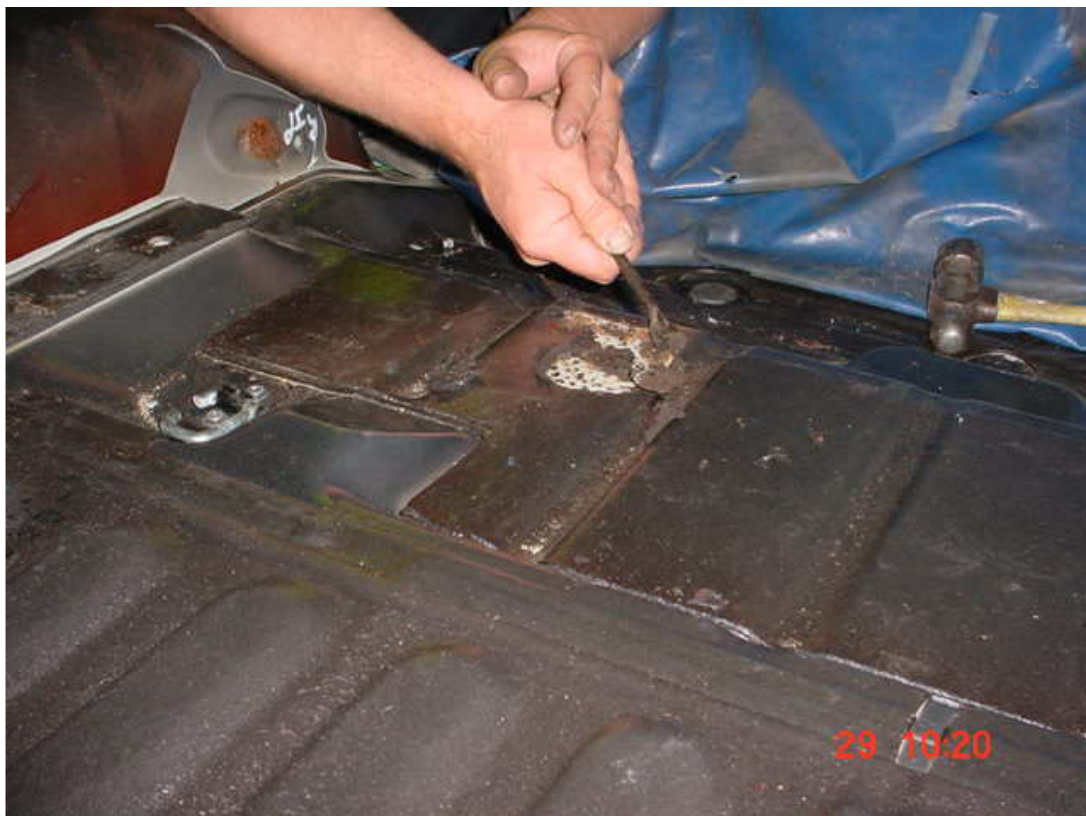
Remove the interior floor coating from underneath the rear seat area.
