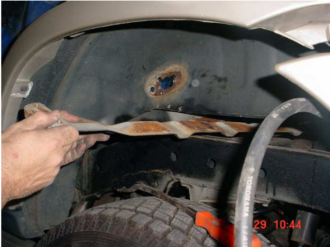
Withdraw the reinforcing plate out the left side of the vehicle.
