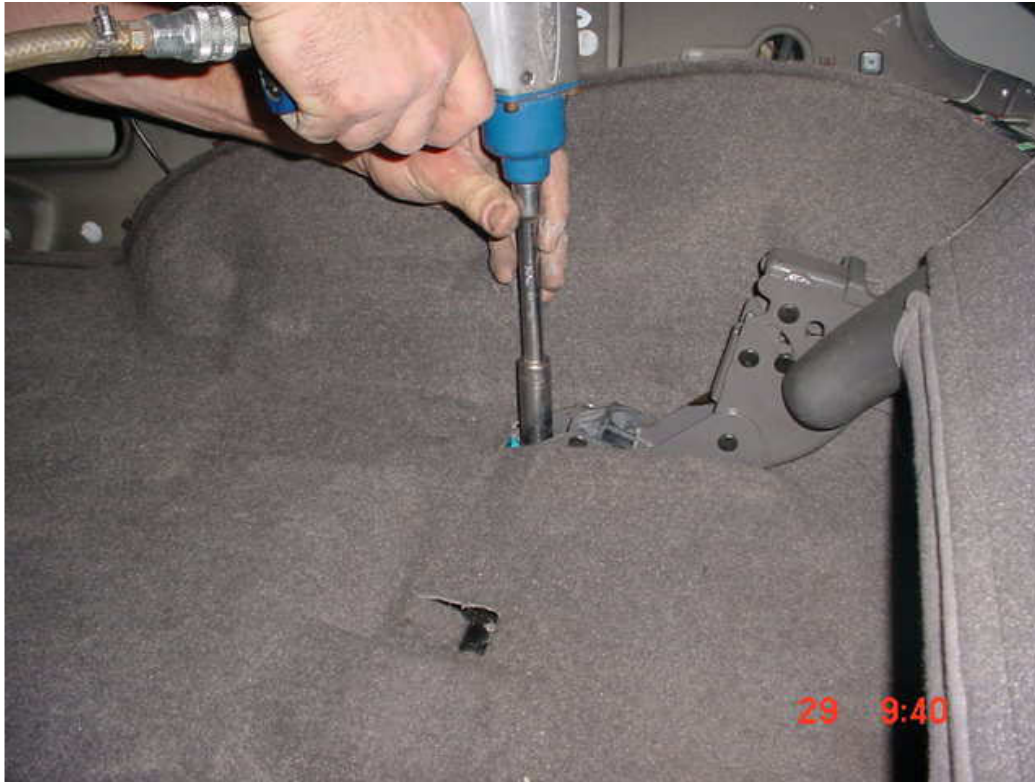
Mistral floor, inside vehicle, remove two bolts from each seat mount.
