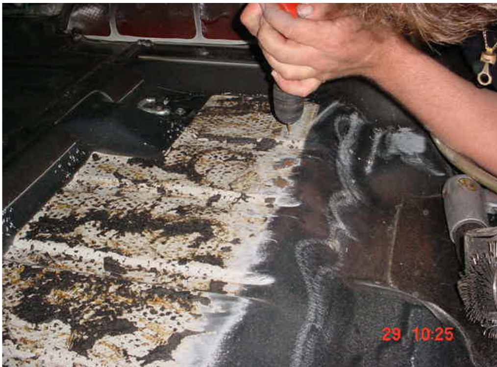
Interior of vehicle floor after wire-wheel cleanup, spot-welds are drilled 2 mm through the central floor section and reinforcing plate, (2 layers).
