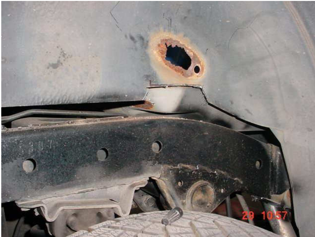
The wheel arch panel has been cut flush with the floor.
