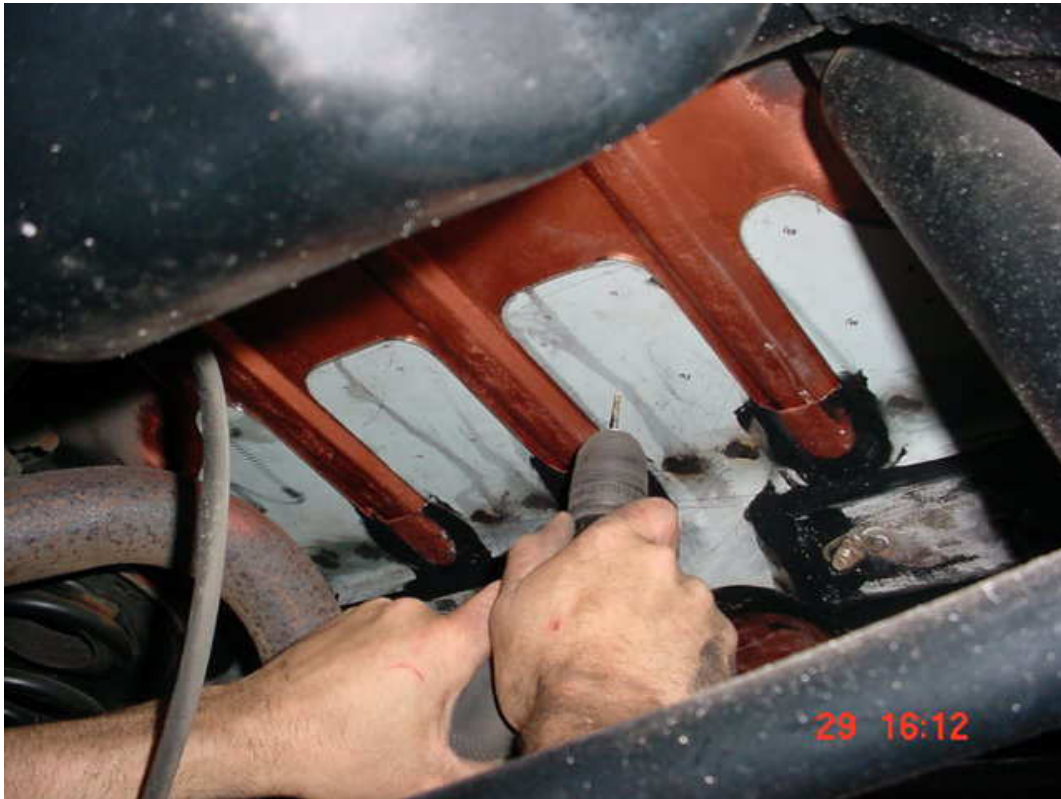
From underneath the vehicle, drill sixteen 2 mm (1/8") holes through the floor, AI using the pre-cut pilot holes in the loadbar.
