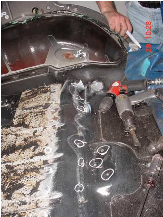
The spot-welds have been marked, there are a total of about 30 including 3 each side beside the wheel arches.
