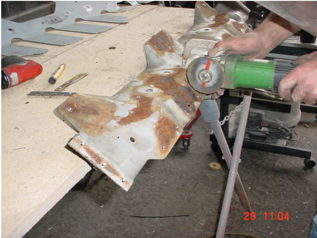
Clean up the reinforcer plate to bare metal using a grinder and/or wire wheel.
