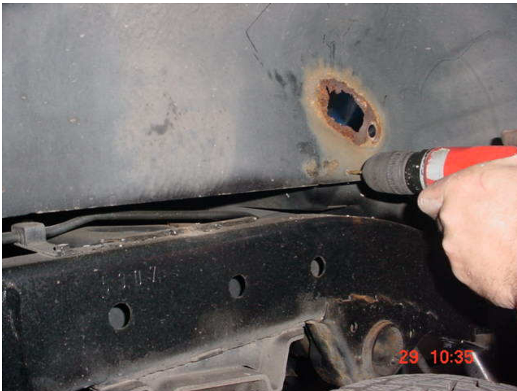
From inside the wheel arch, drill a 2 mm hole through each of three spot-welds below the seatbelt anchorage, through the wheel-arch panel and the reinforcing plate (2 layers), followed by 8 mm through the wheel-arch panel only (1 layer). Note: the seatbelt anchorage plate would normally still be present (see next picture I).
