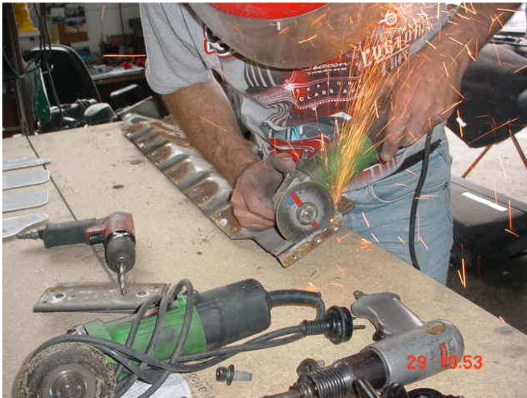
Grind off the two downturned ends on the reinforcing plate. Keep them for use as templates (see photo N).
