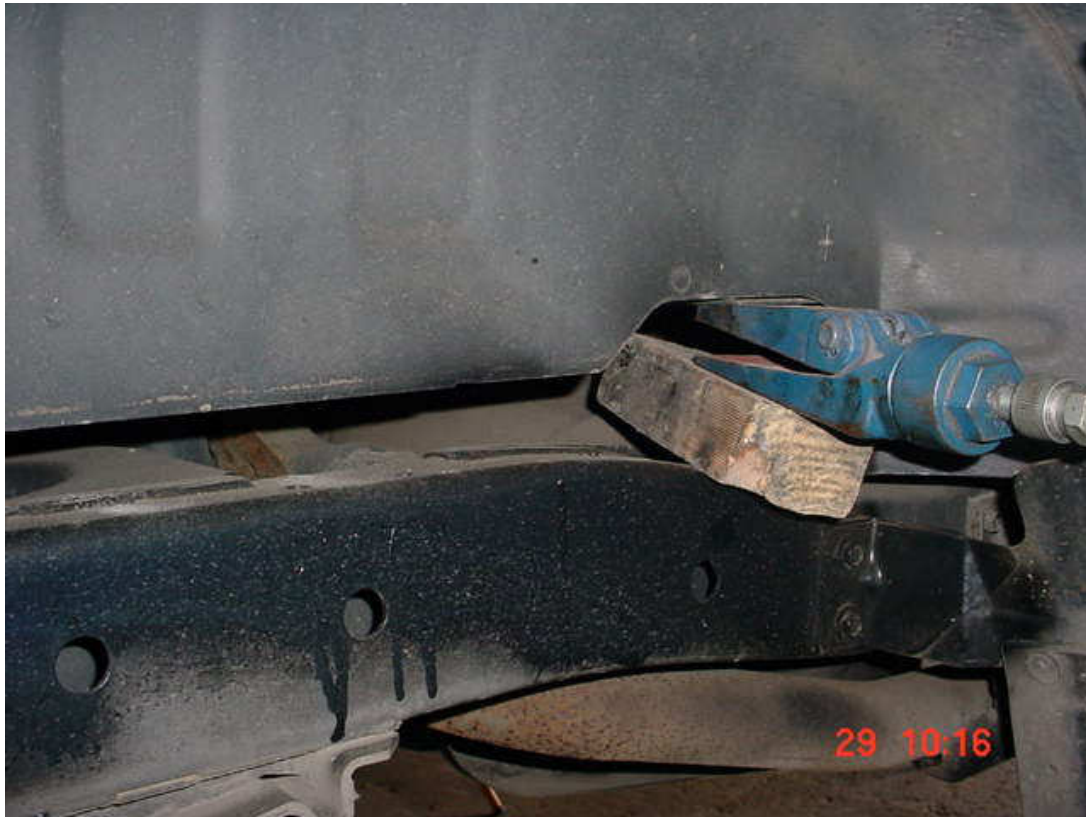
Lift the body from the chassis after removal of the 6 body mounting bolts. Note the rear bumper clip will pop out as the bumper is chassis mounted.
