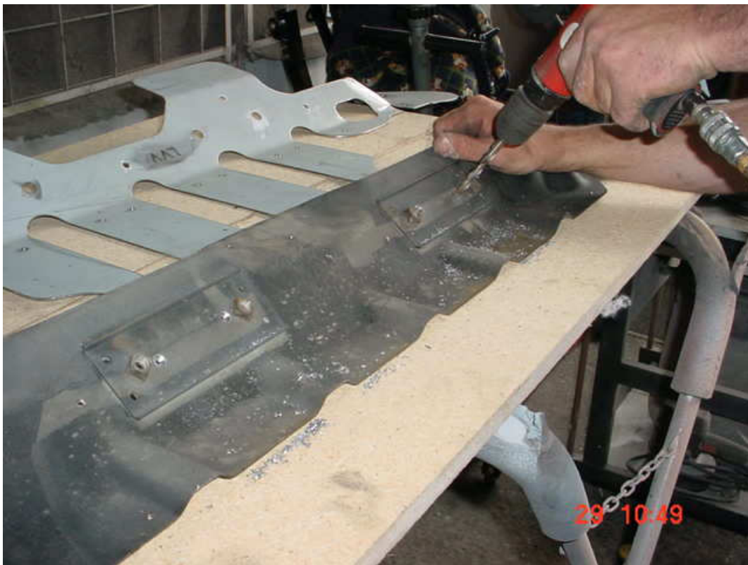
The spot-welds holding the two seat anchorages to the reinforcing plate are drilled through 2mm (both layers) then 8 mm through the seat anchorage plate only (1 layer). Remove the two plates.
