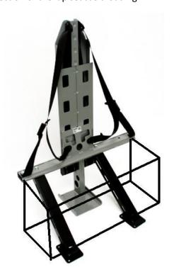
The seat back of an unstressed or lap-stressed seat is ordinarily required to have proof that it can withstand a load of 900N per occupant. In the case of a motorhome rear seat, this can be assessed subjectively. In this case, item 3 of formset FS030 should refer to this LVVTA Information Sheet as justification.
