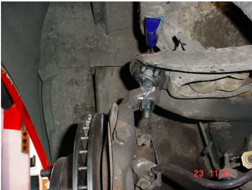
This picture of an XY Falcon with the 4-bolt 'WJ Automotive' balljoint is at the limit of suspension travel due to the balljoint reaching its maximum angular movement. About 25 mm more suspension travel is required to contact the bump-stop.
