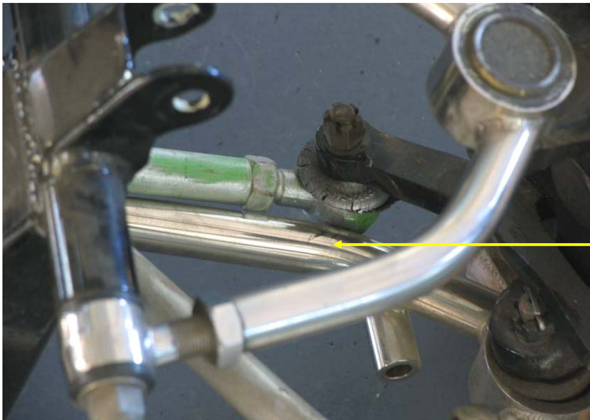
Image 36 – This Image shows the steering tie rod adjusted to demonstrate the possibility of tie rod interference with the suspension arms.
