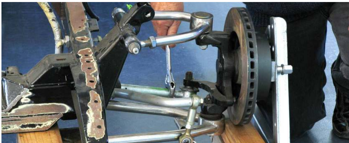
Image 25 - Adjust the tie rods to give a nominal toe of zero.
