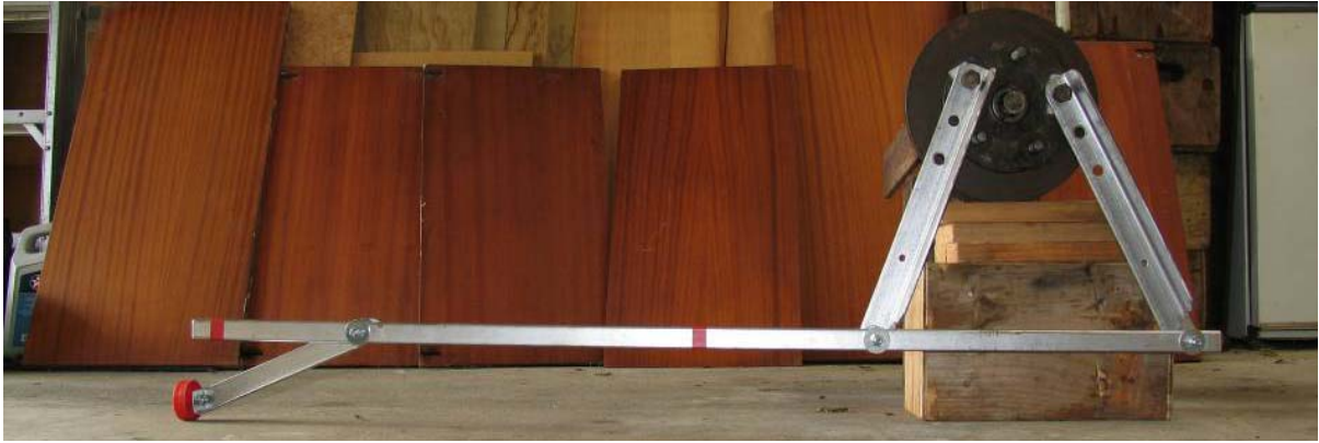
Image 45 - Measuring bars with the droop bracket at the front end which allows for height levelling before measuring. (At nominal ride height)
