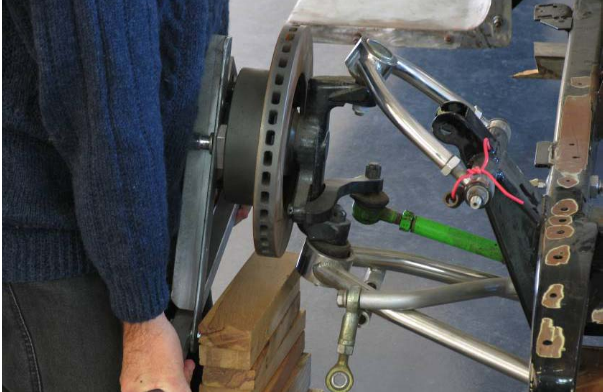
Image 29 - Lift the suspension to ensure the suspension arms will travel further than the minimum coil-over shock length. This is to ensure there is more travel available before the suspension joints bind. Complete this check on both sides.
