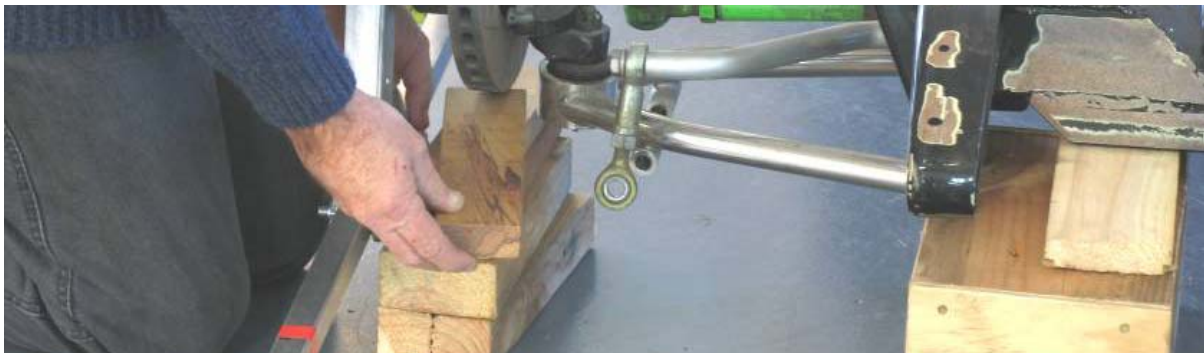
Image 27 - Lift and block the hubs up 20 or 25mm on both sides.
