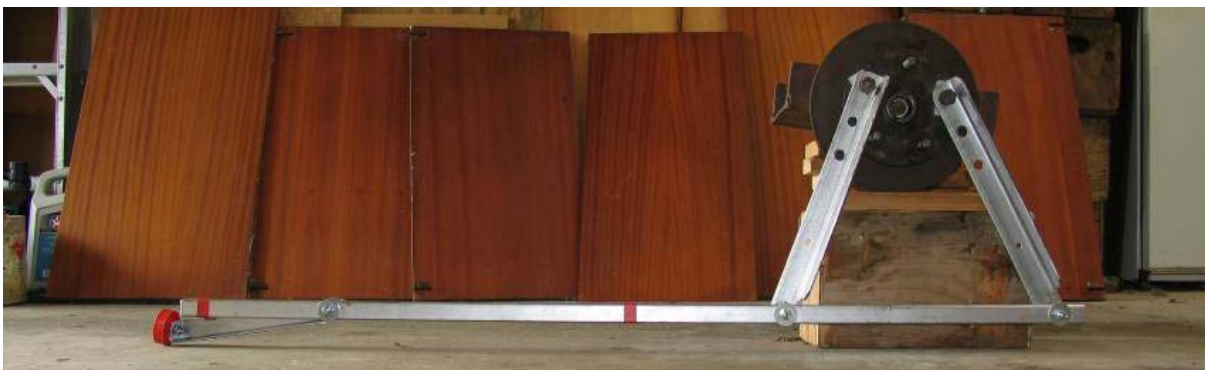
Image 44 - Measuring bars with the droop bracket at the front end which allows for height levelling before measuring. (At full droop)
