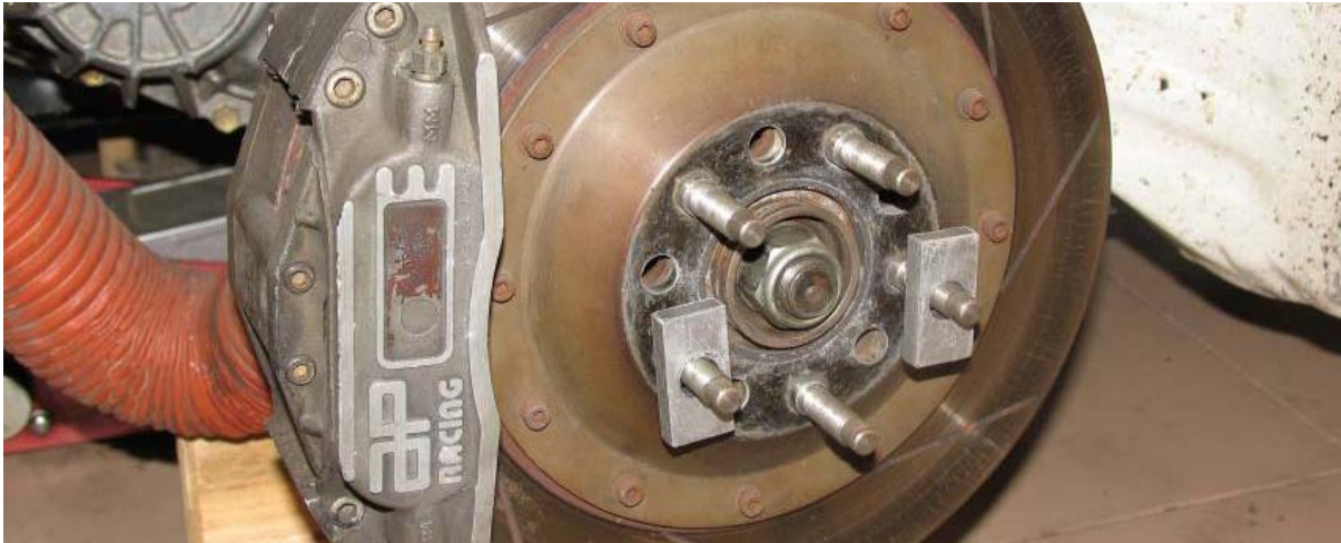
Image 39 - Spacers fitted to hubs.
