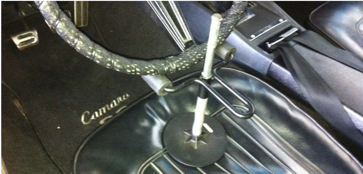
Image 21 – locking the steering. A tool such as this is available from automotive equipment suppliers.
