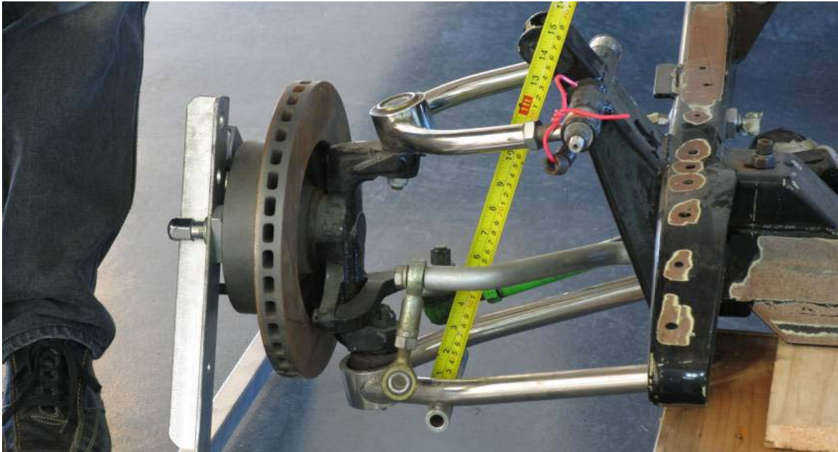
Image 31 - Suspension arms down at full droop.
