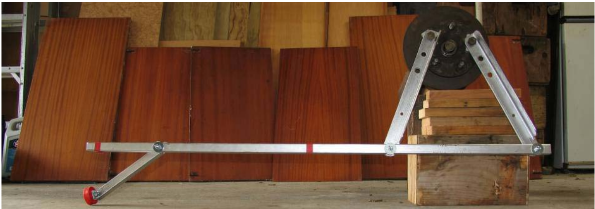
Image 46 - Measuring bars with the droop bracket at the front end which allows for height levelling before measuring. (At full compression)
