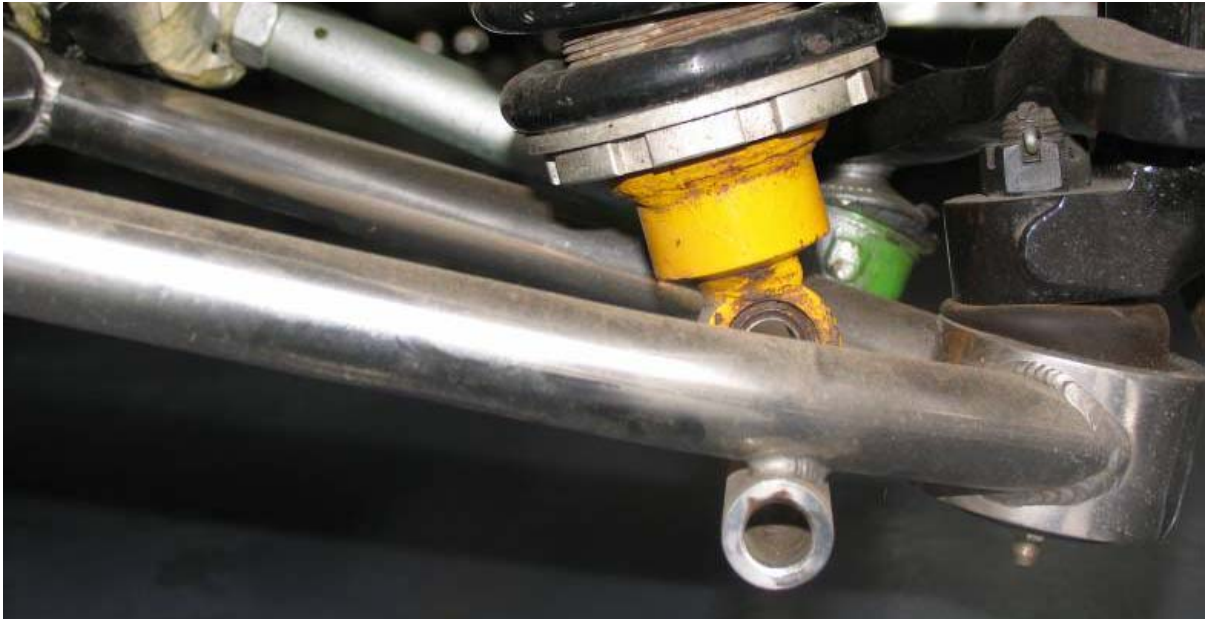
Image 11 - shock fitted at top mount showing suspension with further travel than the shock length, which is needed to prevent ball joint binding.
