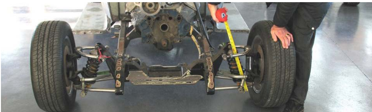
Image 5 - measuring length of coil-over shocks from top and bottom mounting points at nominal ride height.
