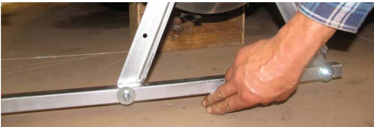
Image 41 - Showing gap below bars and floor.
