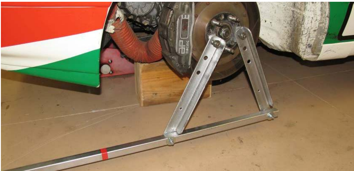
Image 40 - Bump-steer swing-check measuring bars fitted.
