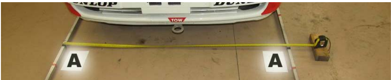
Image 43 - Measure across and under the bumper, spoiler or fenders A to A, and then B to B.
