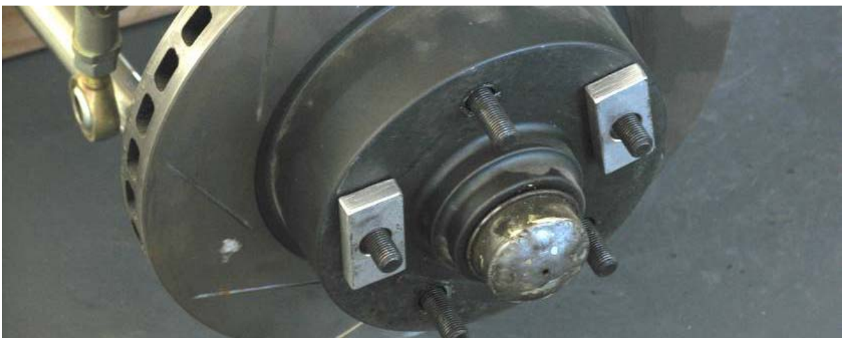
Image 15 - preparing for fitting of the bump-steer swing-check measuring bars, showing spacers fitted to two wheel studs first.
