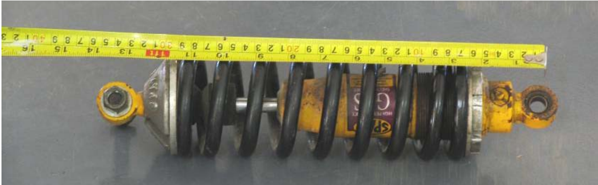
Image 13 - measure and record fully extended coil-over shock length.
