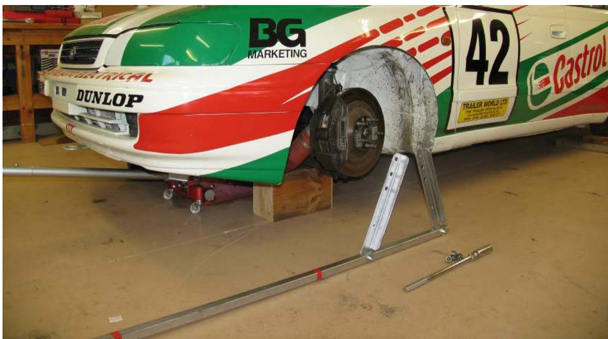
Image 38 - Example of a vehicle with mudguards jacked up to nominal ride height and blocked.
