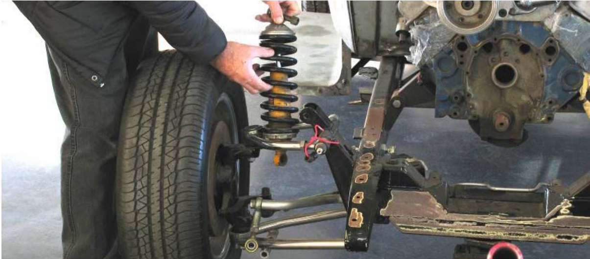
Image 8 - remove coil-over shocks.
