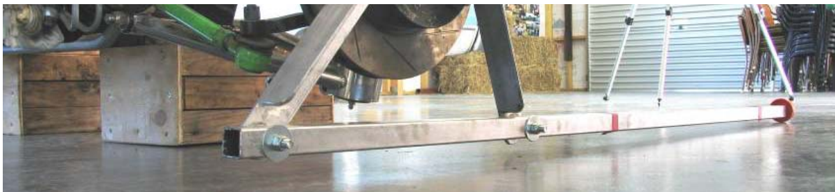
Image 17 - check that the bars are clear of the floor at full suspension droop.
