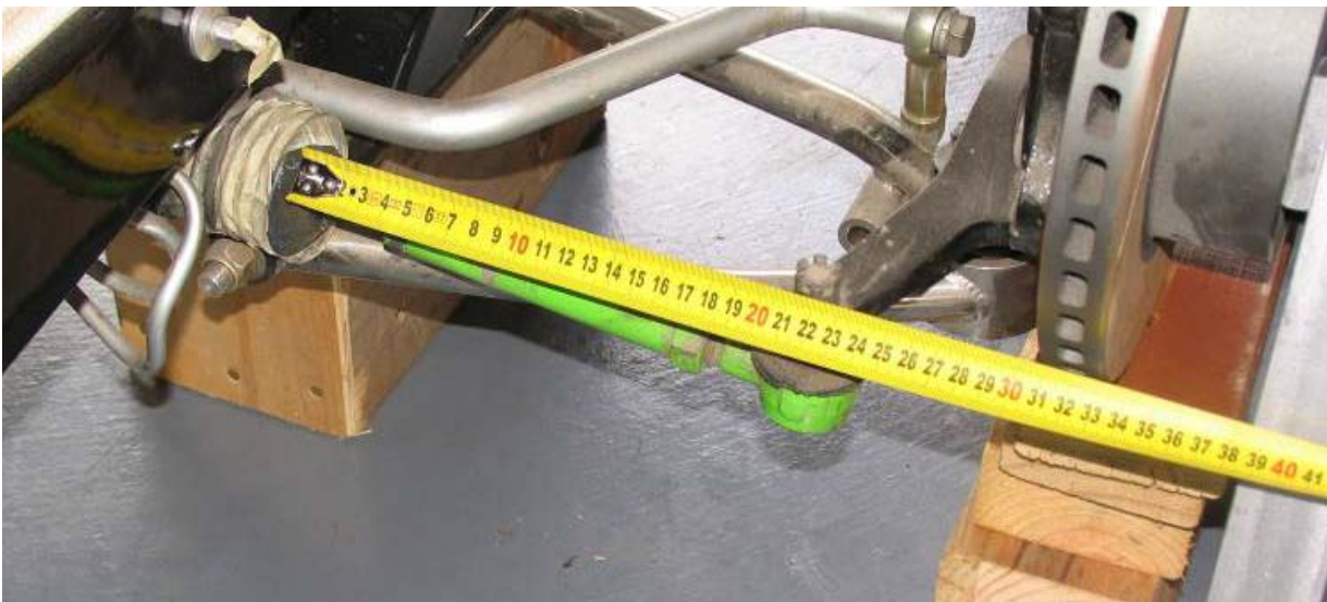
Image 20 - Ensure the tie rods are equal length each side during the adjustment process.
