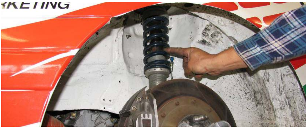
Image 42 - To check this type of strut suspension the coil springs will need to be removed first, and the struts re-installed.
