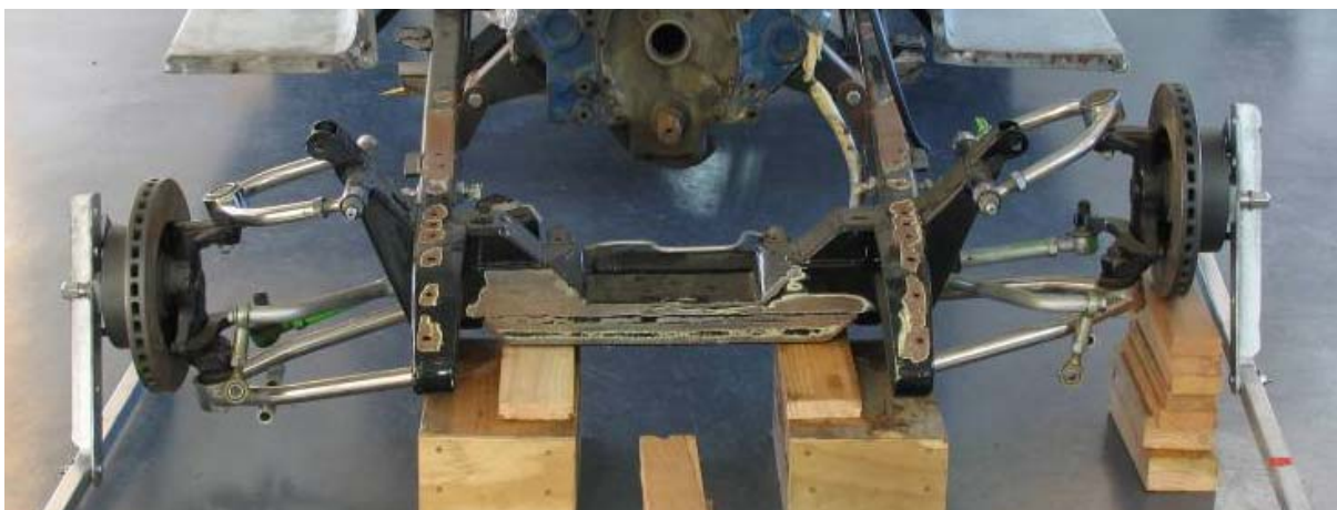
Image 30 – Blocks removed from driver's side showing suspension at full droop.
