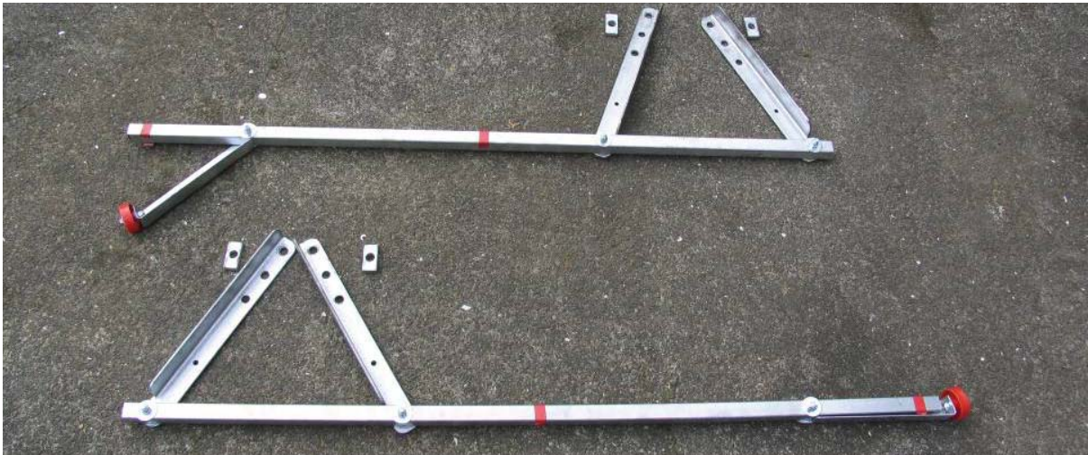
Image 2 – This shows an expanded view of the bump-steer swing-check bars showing the levelling legs and spacers.
