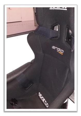
In some cases however, it will not be possible to provide LVV certification for the replacement of the original side-impact airbag-equipped seat with a sports seat. Many modern vehicles have a seatbelt pre-tensioner device attached to the seat, and this device forms part of the frontal impact protection system. LVV requirements preclude any changes to this system until the vehicle has reached 14 years of age.
