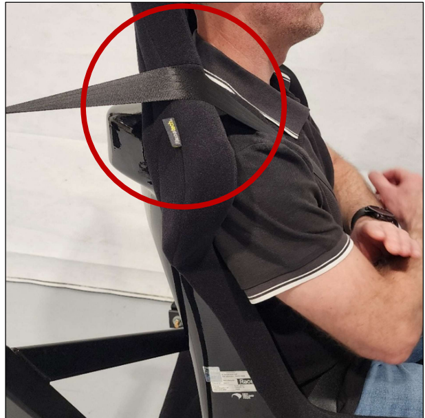
Image 9: The position of the upper seatbelt anchorage in relation to the seat can be crucial when determining whether a seat is acceptable or not. A low seatbelt anchorage (see Image 8) is very unlikely to work correctly with a seat with large shoulder supports (like the one shown in Image 9), as the seatbelt will sit over the seat, rather than the occupant's shoulder.
