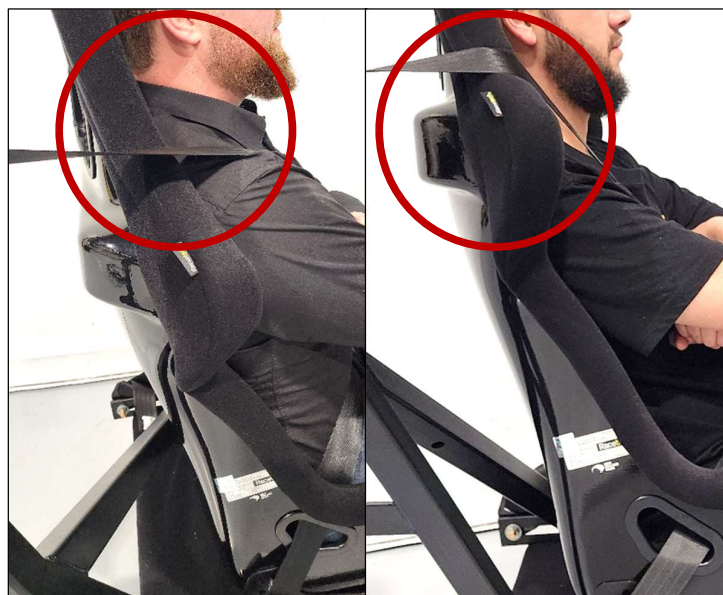
Images 6 and 7: Routing a seatbelt over the head and shoulder restraint 'wing'.
