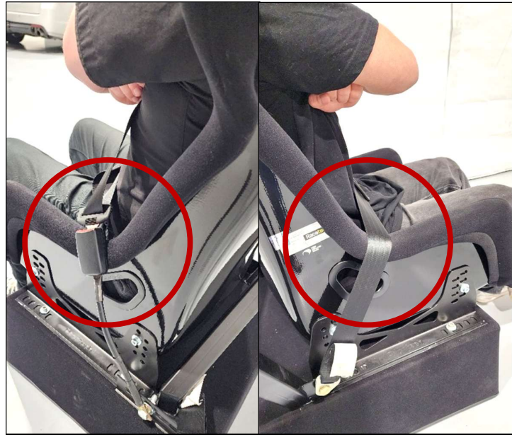
Images 4 and 5: Routing a seatbelt over the seat bolster.
