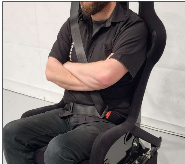
Image 11: Using a 'floppy' fabric webbing-type buckle gives the best chance of positioning the seatbelt correctly on the seat occupant. On this occupant, the buckle sits over the hip, however on a smaller occupant the buckle may sit too high, or too far forward. Note that this fitment is on the borderline of acceptability - the ideal position for the buckle would be lower on the hip, closer to the side of the seat.
