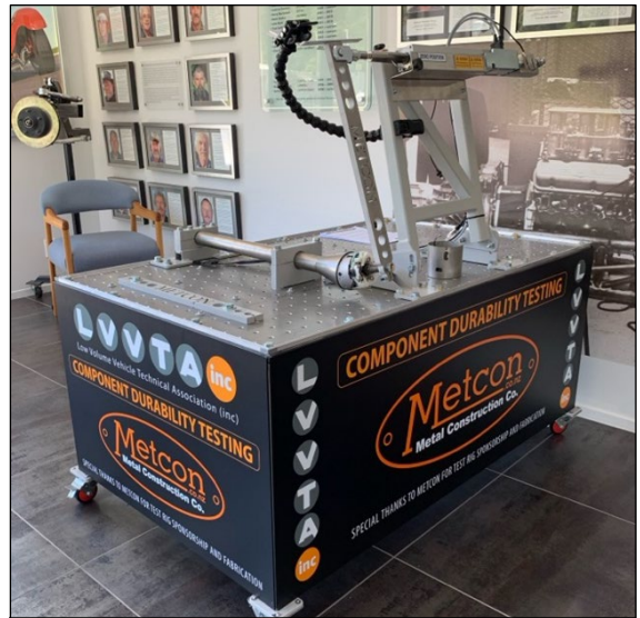
Image 2: LVVTA's custom-built cyclic test rig, with the 'Flaming River'-brand column mounted and ready to begin testing.
