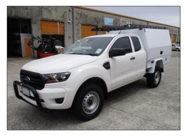
How a vehicle's GVM is rated can depend on things like chassis design and strength, suspension capability, and brake efficiency, as these all influence how much load a vehicle can safely carry.
