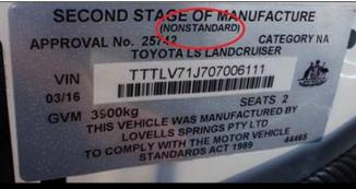
**Left:** This is an example of an acceptable Australian Second Stage of Manufacture compliance label, reproduced from the VIRM. As per <u>Technical Bulletin 13</u>, the plate/label is silver in colour, and has the required information to be accepted as an overseas certification.
