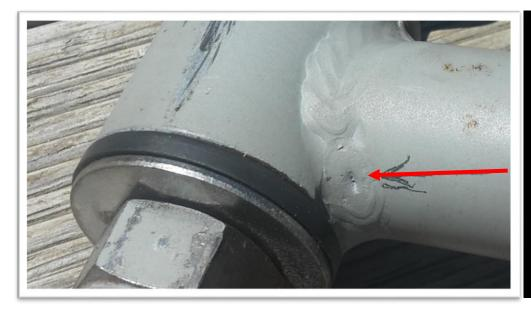
An undesirable 'crater' can be clearly seen in this photograph. Such an imperfection can cause weakness in the weld, and is caused by poor operator techniques in the start/stop regions of
