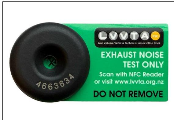
*A vehicle that passes an ONT will, from the 1<sup>st</sup> of October, be fitted with an EDP. This will be accompanied by a green label (above) unless it's also LVV certified and on an EDP, in which case it will have an orange label (below).*
