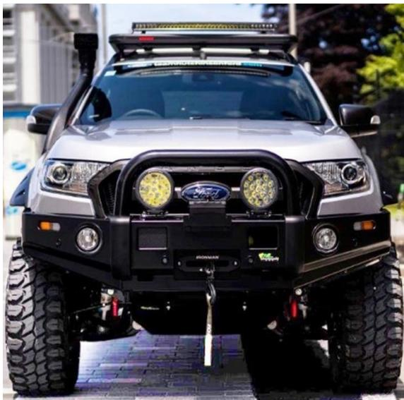
**Image 5.** Aftermarket wheels, tyres, and mudguard extensions. Tyre tread extends further than 25mm outside of the unmodified original body panels, or factory-fitted mudguard extensions: LVV certification **is** required.
