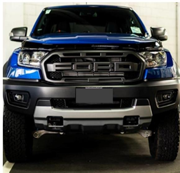
**Image 6.** The Ford Ranger Raptor is factory-fitted with wide steel guards and plastic fender flares. The tyre tread is already 25mm outside of the unmodified original [steel] body panels. Any increase in the outside tread position on this vehicle means that: LVV certification **is** required.
