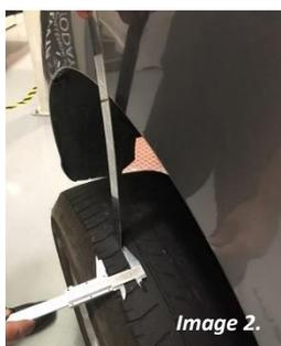
The new wording uses the OE body panel position as a datum point instead of the track so this can be more readily measured.
