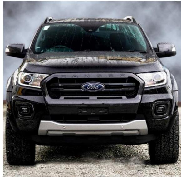
**Image 4.** Aftermarket wheels with aftermarket fender flares, however the tyre tread does not extend by more than 25mm outside of the unmodified original body panels: LVV certification is **not** required.
