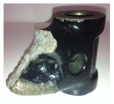
The investigation process had included a metalurgical analysis of a section of the failed axle in order to determine the exact material composition.
