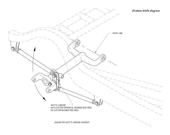
Diagram 3: Watts linkage geometry
