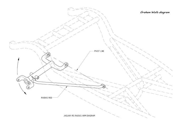
Diagram 2: Radius rod geometry
