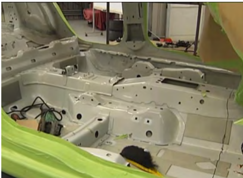
Above: The factory floor, cross members, transmission tunnel, and subframe (chassis) rails were removed.
