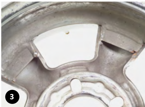
Image 1: Front face of typical copy of an Astro Supreme-brand wheel. Image 2: 'DOT' compliance marking is evident on rim, but that applies only to the rim itself, not the manufactured wheel. Image 3: View of back-face of a poorly designed and assembled 'Supreme' type wheel. Image 4: Weld failures on a copy of an Astro Supreme-brand wheel. Image Source: Photos kindly supplied by Vahry Photography, Parnell, Auckland.
