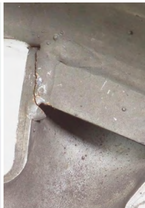
Left: Front face of typical copy of an Astro Supreme-brand wheel. Right: Weld failures on a copy of an Astro Supreme-brand wheel. Image Source: Photos kindly supplied by Vahry Photography, Parnell, Auckland.
