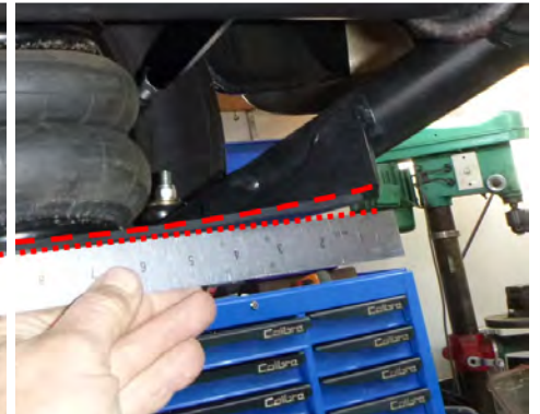
Image 1: A PBFab (Porterbuilt) Chevrolet C10 lower arm showing the cantilever-style ball joint platform design. Image 2: This is an example of a poor weld including craters and incomplete welds at the ball joint end housing. Image 3: This is an example of a Chevrolet C10 truck Ridetech lower control arm, with a visible bend or sag in the air bag mounting platform.
