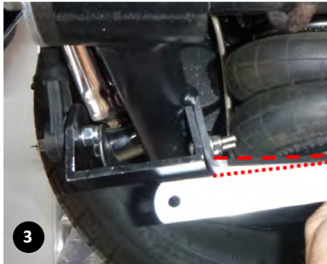
Image 1: A PBFab (Porterbuilt) Chevrolet C10 lower arm showing the cantilever-style ball joint platform design. Image 2: This is an example of a poor weld including craters and incomplete welds at the ball joint end housing. Image 3: This is an example of a Chevrolet C10 truck Ridetech lower control arm, with a visible bend or sag in the air bag mounting platform.
