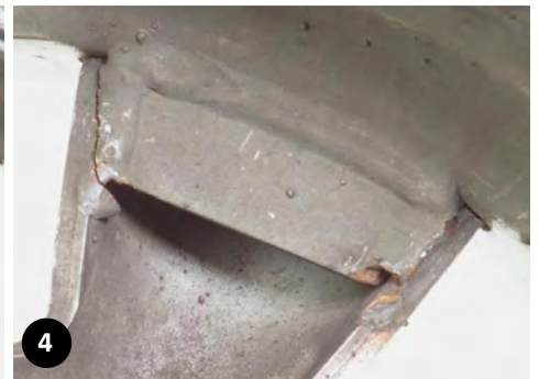
Image 1: Front face of typical copy of an Astro Supreme-brand wheel. Image 2: 'DOT' compliance marking is evident on rim, but that applies only to the rim itself, not the manufactured wheel. Image 3: View of back-face of a poorly designed and assembled 'Supreme' type wheel. Image 4: Weld failures on a copy of an Astro Supreme-brand wheel. Image Source: Photos kindly supplied by Vahry Photography, Parnell, Auckland.
