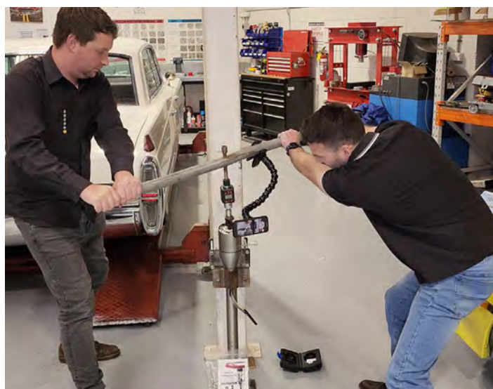
Above: LVVTA technical staff members Dylan Mathieson (left) and Andrew McGregor conduct the maximum load test on an 'Ididit'-brand tilt column.
