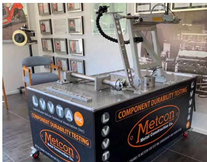
Above: LVVTA's custom-built cyclic test rig, with the 'Flaming River'-brand column mounted and ready to begin testing.
