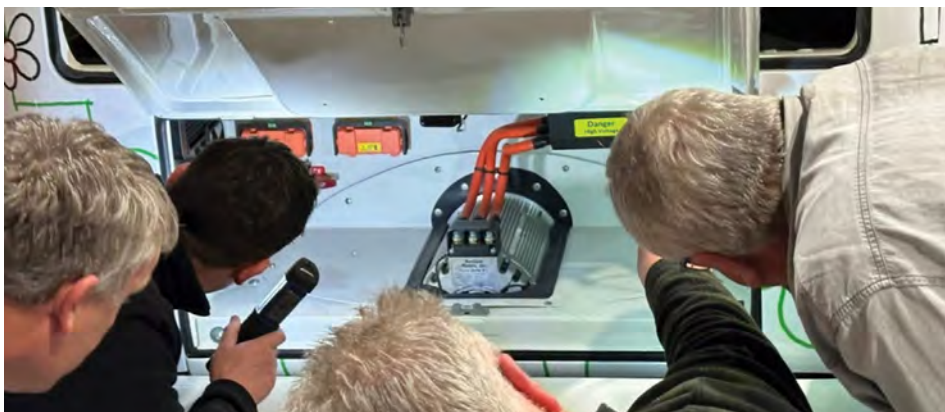
Top left: Industry experts, LVV Certifiers and LVVTA staff discuss changes to the LVV Electric & Hybrid Vehicles Standard to bring it in line with current technology and trends. Top right: Attendees inspect the main battery pack installation under the converted VW Kombi. Bottom: Very tidy 'engine' bay with the electric motor replacing the VW Kombi's ICE. Photo courtesy of Vahry Photography, Parnell, Auckland.
