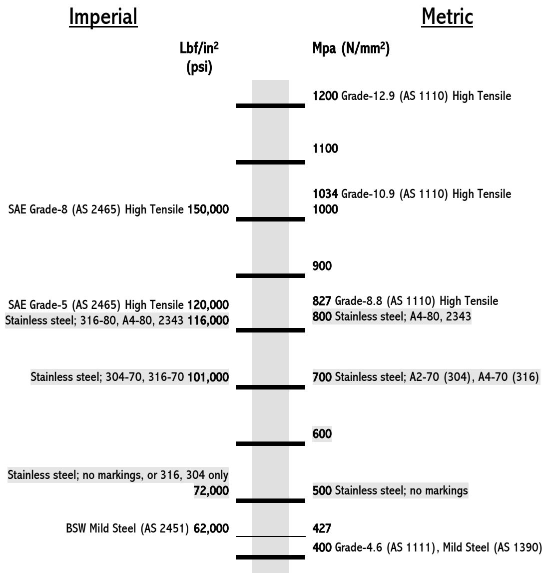
**Table 18.4 Fastener tensile strength comparison guide table**
