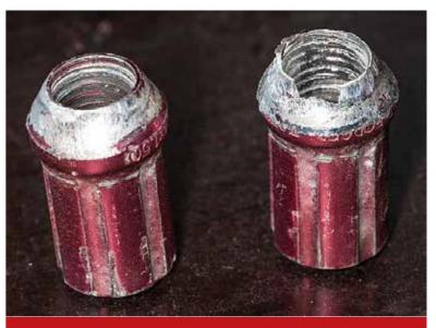
These aluminium wheel nuts are part of a set that failed, resulting in a wheel detaching from the vehicle the vehicle being involved in a head on collision, where the driver sustained fatal injuries.
