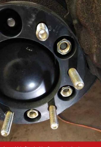
Any vehicle fitted with aftermarket wheel spacers or adaptors requires LVV Certification before a Warrant of Fitness can be issued. Part of the inspection process is to ensure thread engagement meets requirements. The example shown here has dangerously-low thread engagement.
